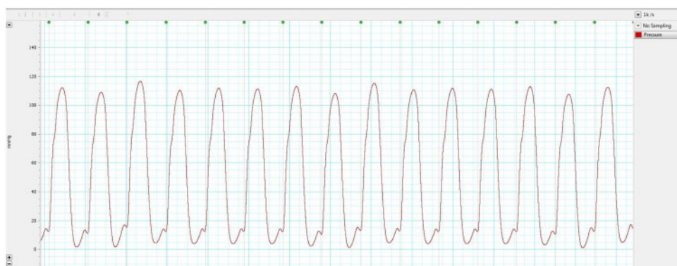
Figure 2: Sample of right ventricular pressure signal obtained using the technique described in the article.
